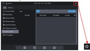
Click "Device search" in the left menu and "Auto topology" in the right area. The centralized controller will start to obtain information about the refrigerant system connected to the centralized controller and automatically construct the topological relationship. After this, the interface will appear as follows:
