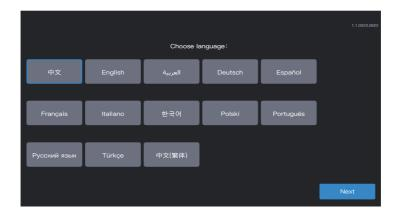
When the centralized controller is powered on for the first time, select the display language of the centralized controller.
