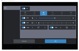
Note: If the IDU does not support single attribute setting, "keep" cannot be selected for any parameter. (Consult the technical staff about whether the specific model supports a single attribute) Note: The control parameters displayed on the interface may exceed the actual controllable parameters of the IDU. When this parameter is selected, the actual IDU does not operate.
